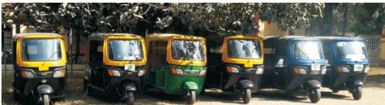
Hydrogen (stored in hydride) fueled three wheeler demonstration fleet at Hydrogen Energy Centre BHU
